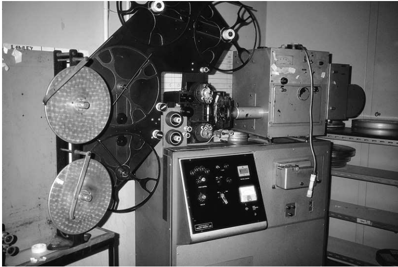
Figure 13.4 A 35 mm Neilson–Hordell step contact register printer, with a 1970s additive lamphouse (Soho Images, London)
