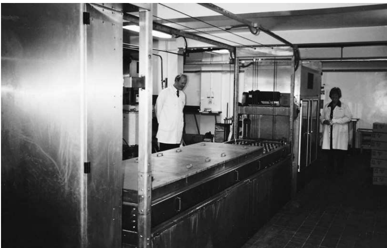
Figure 16.5 A modern black and white print film processor capable of 150 feet per minute (2700 m/h) at Henderson's Film Laboratories, London
