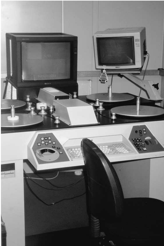
Figure 14.1 A Filmlab Colormaster video analyser at Soho Images in London – a modern closed circuit colour telecine and display unit for grading colour negatives
