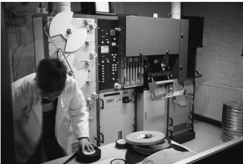
Figure 13.10 A Debrie TAI Printer, 35 mm step optical with a total immersion wet gate, additive lamphouse and variable pitch pull down for shrunken film (Cinemathèque Royale de Belgique, Brussels)
