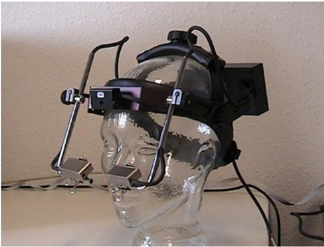
Figure 6.5 A head-mounted eye-tracking system. With permission of William C. Schmidt, SR Research Limited, http://www.sr-research.com/EL_II.html
