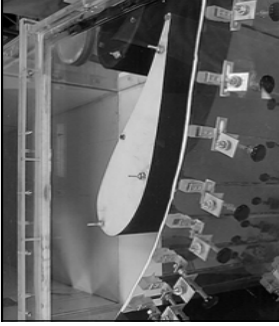
Figure 4. Large-scale turbine vane in wind tunnel.
