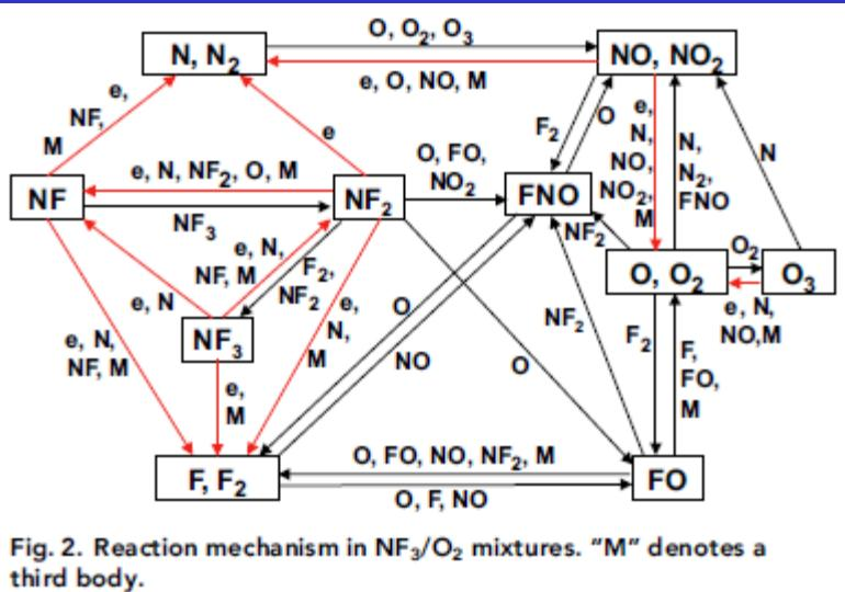
Fig. 2. Reaction mechanism in  $\text{NF}_3/\text{O}_2$  mixtures. "M" denotes a third body.
