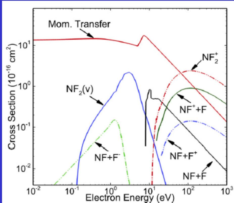
Fig. 12. Some cross sections used for the processes depicted in Fig. 2. The data for electron collisions with  $\text{NF}_2$ , including momentum transfer, vibrational excitation ( $v$ ), and dissociation into combinations of various molecular ions were generated by Tennyson and collaborators (42) with the UK molecular R-matrix codes (43).
