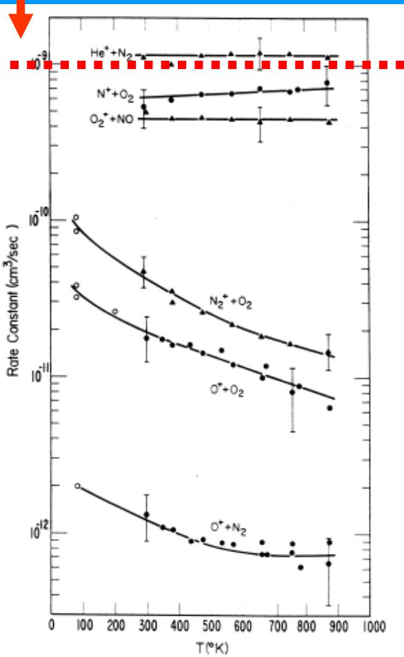
$$k_{\text{col}} = \langle v \rho \rangle \sim \langle v \rangle / \langle v \rangle = \text{const.}$$
