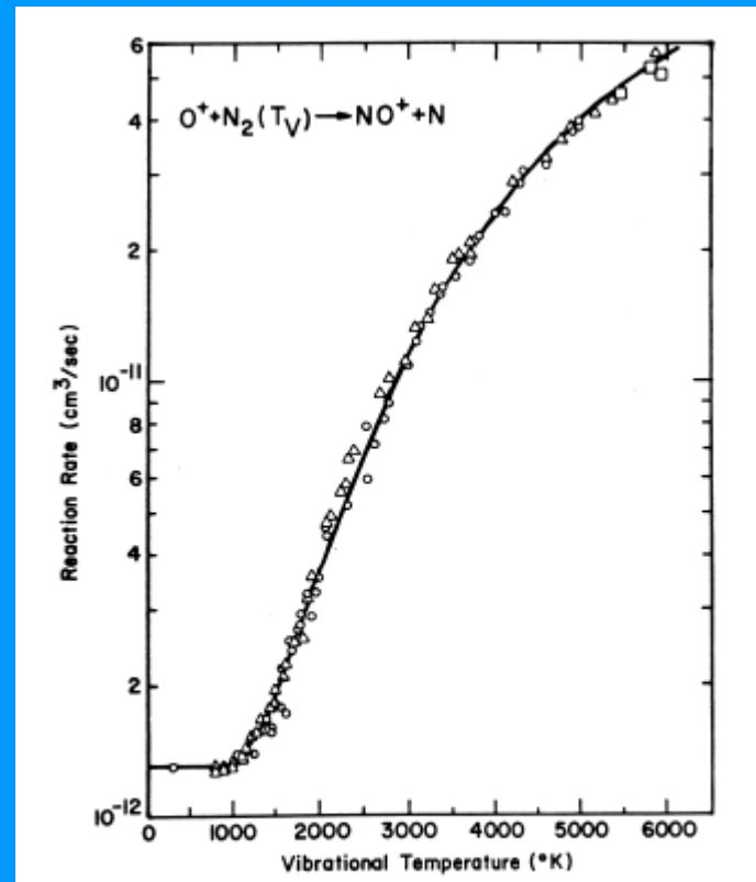
Fig. 12. Measurements of the variation of the rate coefficient for the reaction of  $\text{O}^+ + \text{N}_2 \rightarrow \text{NO}^+ + \text{N}$  with the vibrational temperature of  $\text{N}_2$  [16].
