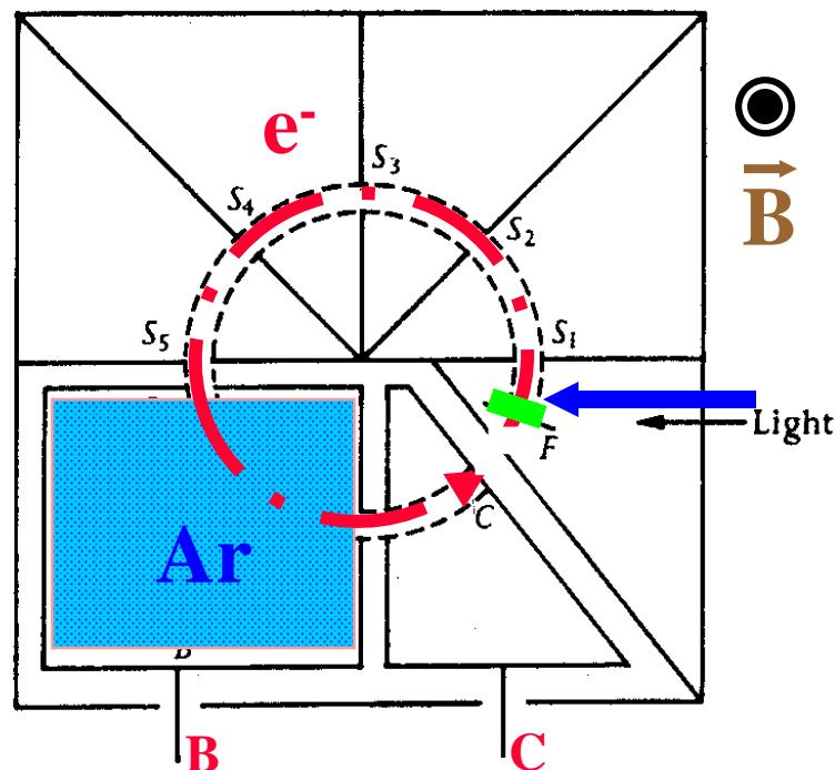
FIG. 1.1. Ramsauer's apparatus for measurement of collision cross-sections.
