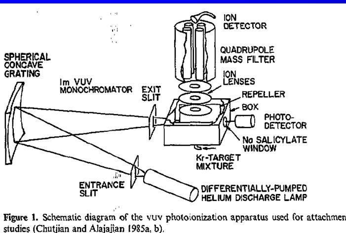
Figure 1. Schematic diagram of the vuv photoionization apparatus used for attachment studies (Chutjian and Alajajian 1985a, b).
