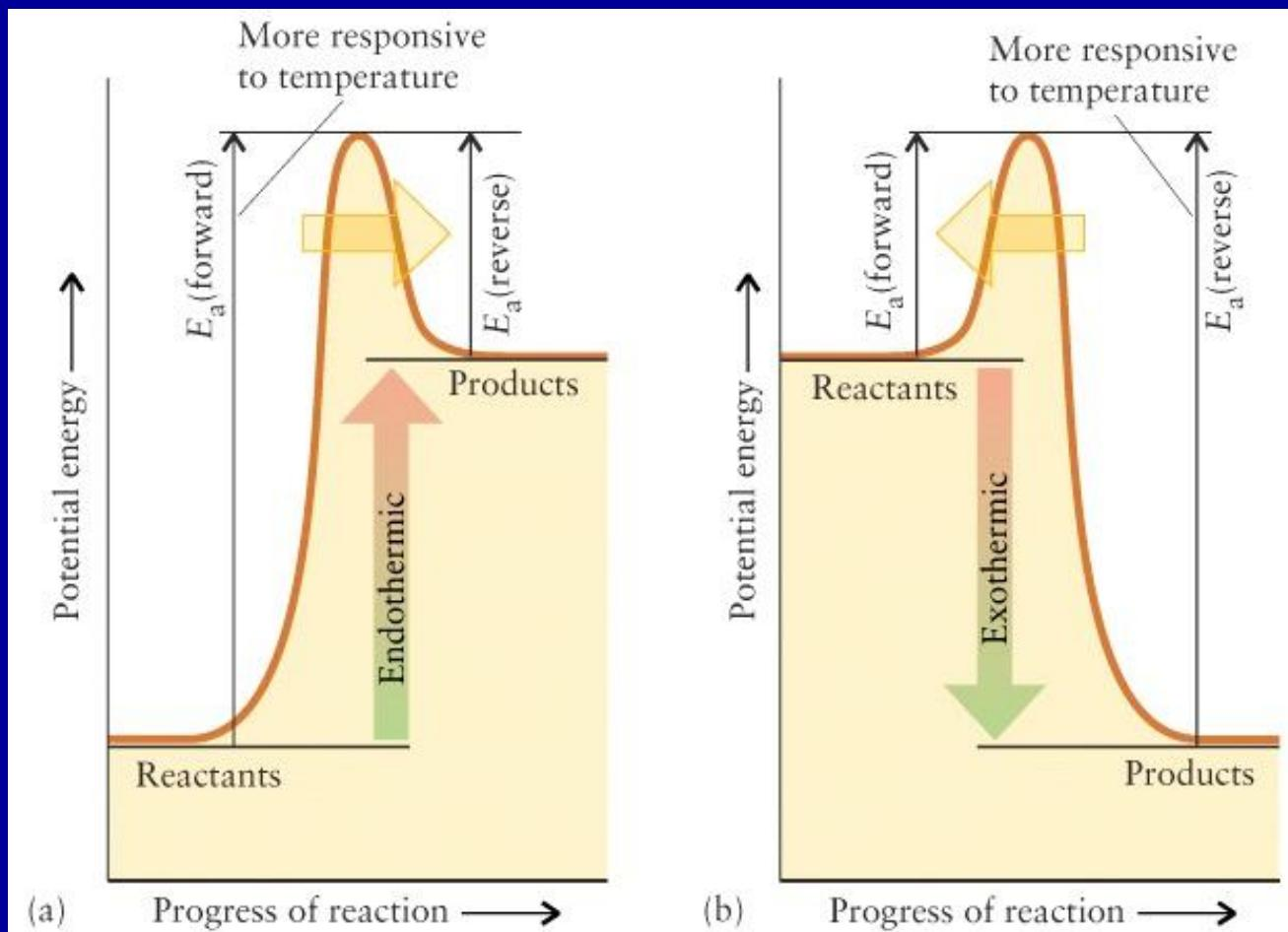
**Endothermic reaction:  $E_a(\text{forward}) > E_a(\text{reverse})$**
