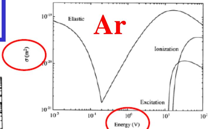
3. Ionization, excitation and elastic scattering cross sections for electrons in argon gas (compiled by Vahedi, 1993).
