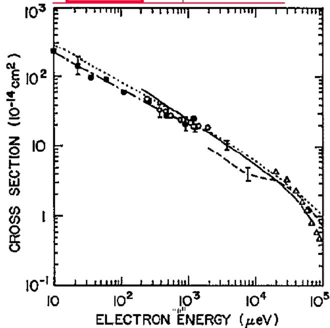
Figure 2. Cross section for electron attachment to SF<sub>6</sub>. ■,  $\bar{\sigma}_e$ -K(np); — · —,  $\bar{\sigma}_e(\nu)$ -K(np) (Ling *et al* 1992). ○,  $\bar{\sigma}_e$ -Rb(ns) (Zollars *et al* 1985); —, free electrons (Klar *et al* 1992a, b); - - -, free electrons (Chutjian and Alajajian 1985); △, free electrons (Pai *et al* 1979, Chutjian and Alajajian 1985a); ---, theory (Klots 1976).
