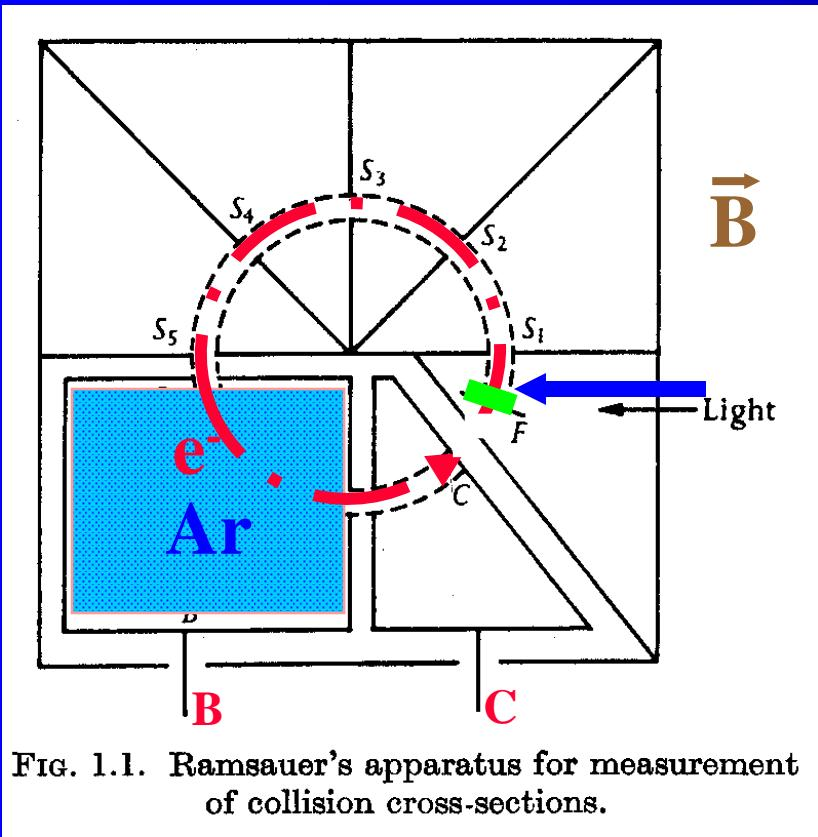
FIG. 1.1. Ramsauer's apparatus for measurement of collision cross-sections.
