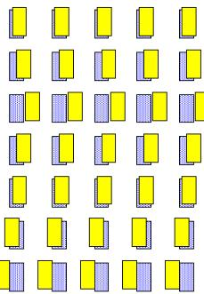
A plasma oscillation: displaced electrons oscillate around fixed ions. The wave does not necessarily propagate.
