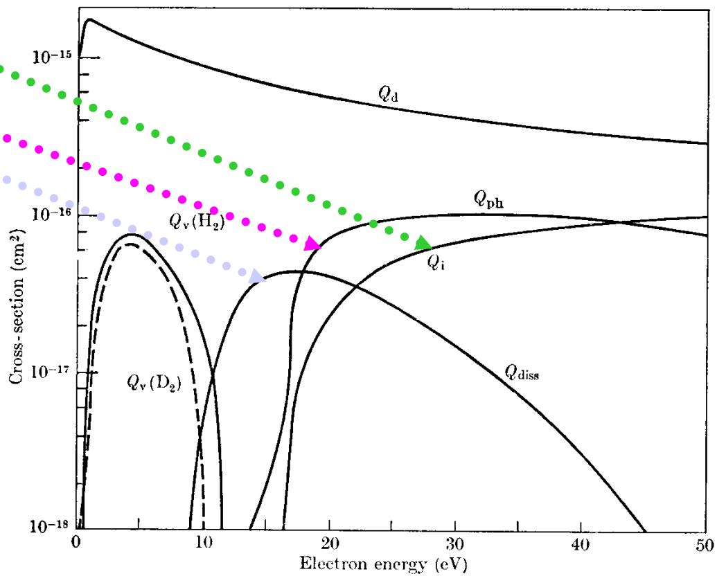
FIG. 13.37. Cross-sections assumed by Engelhardt and Phelps in their analysis of swarm data in H<sub>2</sub> and D<sub>2</sub> for electrons of characteristic energy greater than 1 eV.  $Q_d$  momentum-transfer cross-section,  $Q_i$ , ionization cross-section,  $Q_{diss}$  dissociation cross-section,  $Q_{ph}$  photon excitation cross-section,  $Q_v$  vibrational excitation cross-section (— H<sub>2</sub>, - - - D<sub>2</sub>).
