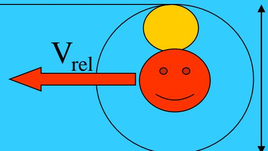
$$I(t) = I_0 \exp(-\nu_{coll} t) = I_0 \exp(-\sigma n v_{rel} t)$$
