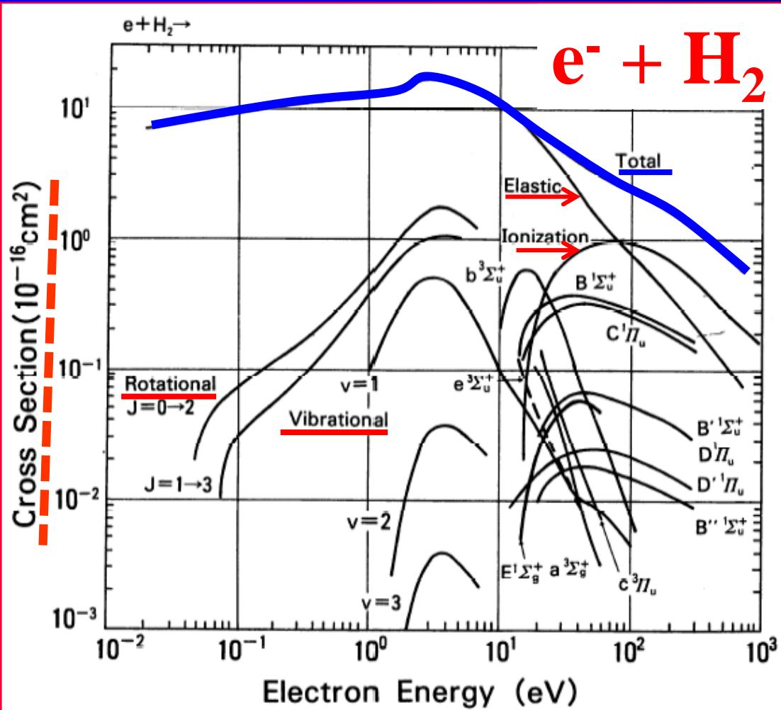
FIG. 2. Comparison of cross sections for various collision processes in neutral H<sub>2</sub>. Also for comparison, cross sections of ionization of atomic hydrogen are shown. These data are taken at room temperatures.
