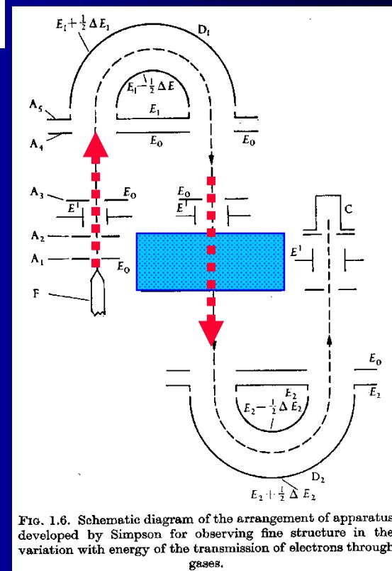
FIG. 1.6. Schematic diagram of the arrangement of apparatus developed by Simpson for observing fine structure in the variation with energy of the transmission of electrons through gases.
