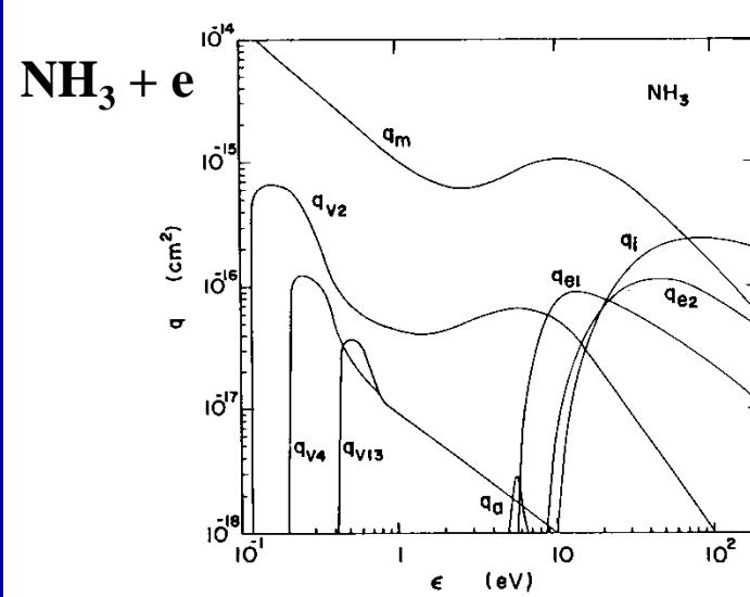
Fig. 6. Electron collision cross-section set for  $\text{NH}_3$  (1986).
