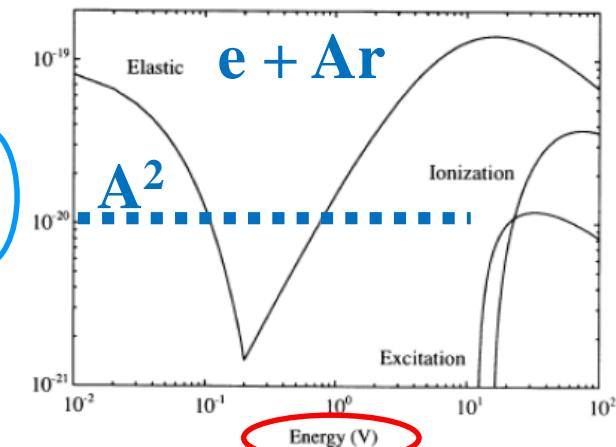
3. Ionization, excitation and elastic scattering cross sections for electrons in Ar (compiled by Vahedi, 1993).
