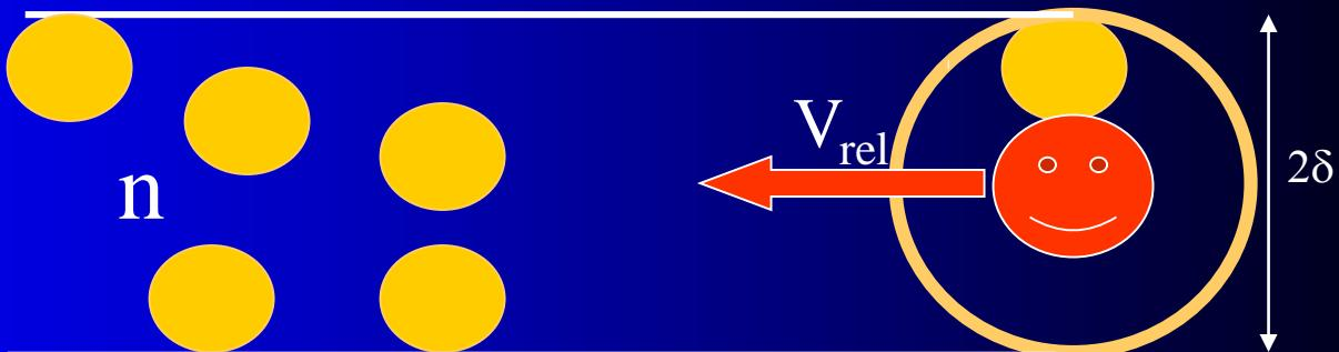
$$I(t) = I_0 \exp(-\nu_{coll} t) = I_0 \exp(-\sigma n V_{rel} t)$$
