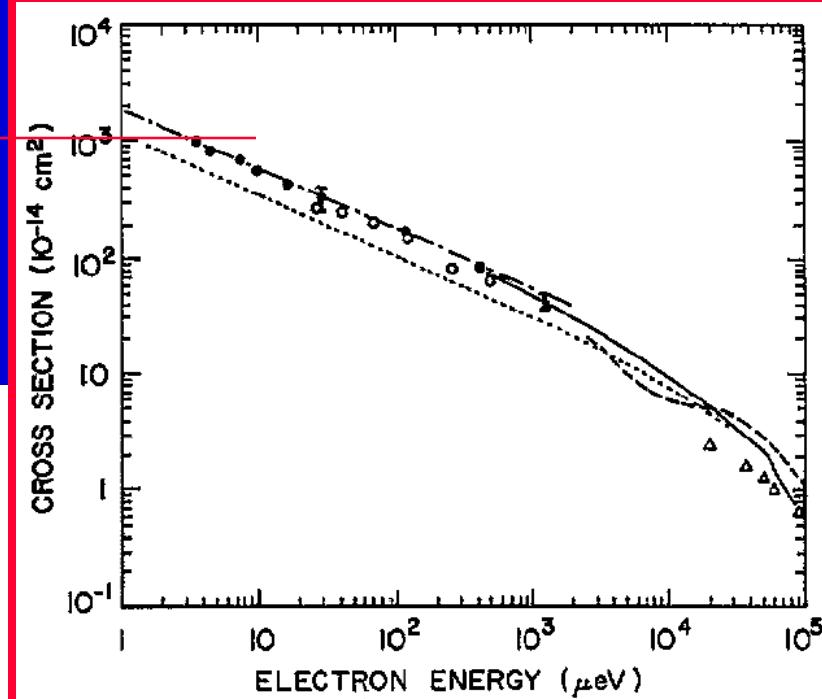
Figure 3. Cross sections for electron attachment to CCl<sub>4</sub>. ●,  $\bar{\sigma}_e$ -K(np); — · —,  $\bar{\sigma}_e(\nu)$ -K(np) (Frey *et al* 1994b); ○,  $\bar{\sigma}_e$ -K(np) (Ling *et al* 1992); —, free electrons (Hotop 1994); - - -, free electrons (Orient *et al* 1989); △, free electrons (Christodoulides and Christophorou (1971)); ---, theory (Klots 1976).
