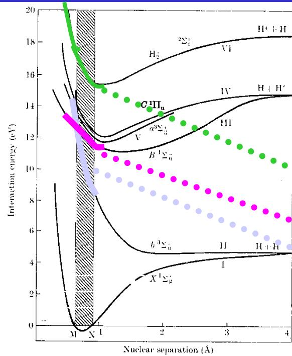
FIG. 13.1. Potential energy curves for electronic states of H<sub>2</sub> and H<sub>2</sub><sup>+</sup> lying within 20 eV of the ground state.
