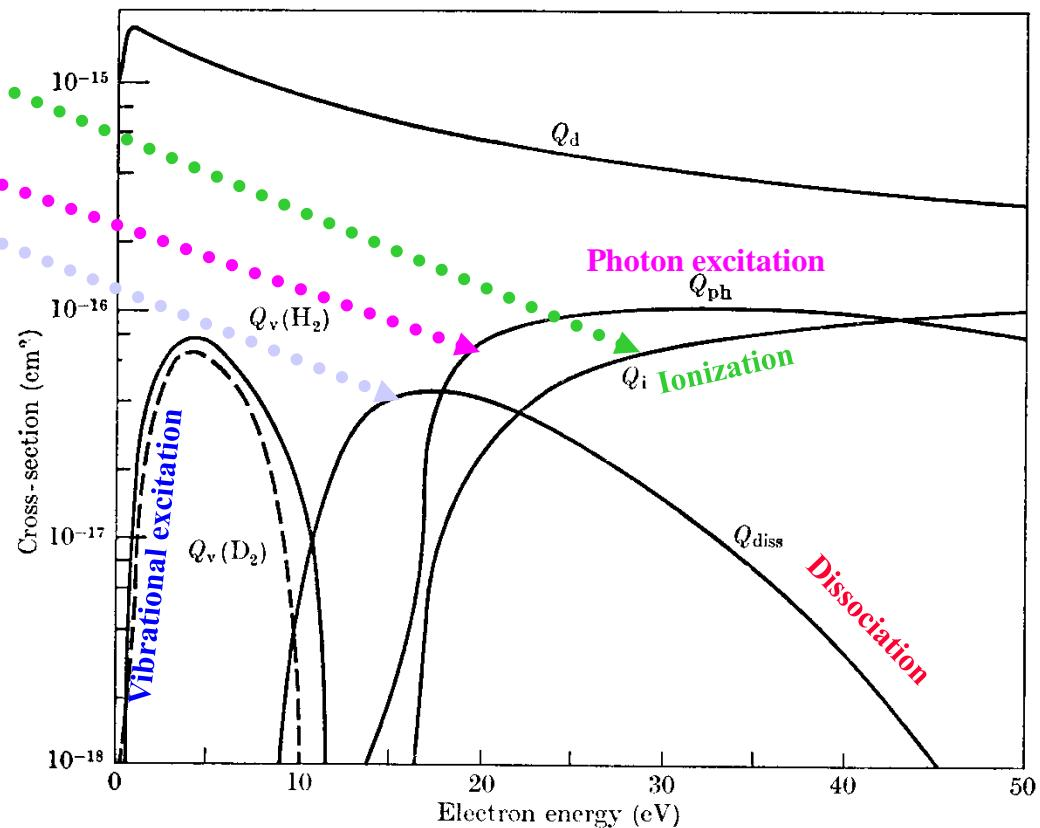
FIG. 13.37. Cross-sections assumed by Engelhardt and Phelps in their analysis of swarm data in H<sub>2</sub> and D<sub>2</sub> for electrons of characteristic energy greater than 1 eV. Q<sub>d</sub> momentum-transfer cross-section, Q<sub>i</sub>, ionization cross-section, Q<sub>diss</sub>, dissociation cross-section, Q<sub>ph</sub>, photon excitation cross-section, Q<sub>v</sub>, vibrational excitation cross-section (— H<sub>2</sub>, - - - D<sub>2</sub>).
