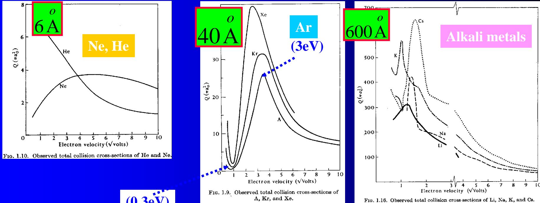
FIG. 1.9. Observed total collision cross-sections of A, Kr, and Xe.
