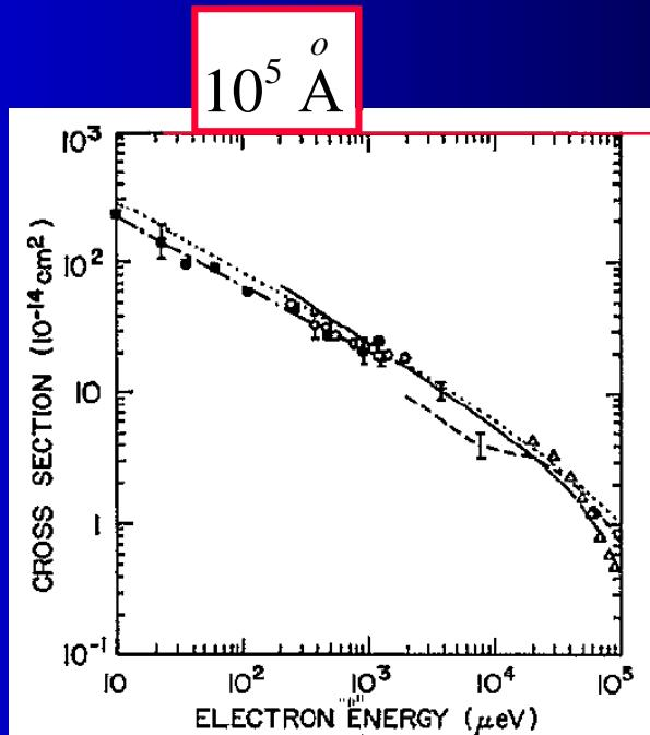
Figure 2. Cross section for electron attachment to  $\text{SF}_6$ . ■,  $\sigma_e - \text{K}(np)$ ; —·—,  $\sigma_e(v) - \text{K}(np)$  (Ling *et al* 1992). ○,  $\sigma_e - \text{Rb}(ns)$  (Zollars *et al* 1985); —, free electrons (Klar *et al* 1992a, b); ---, free electrons (Chutjian and Alajajian 1985); Δ, free electrons (Pai *et al* 1979, Chutjian and Alajajian 1985a); ----, theory (Klots 1976).
