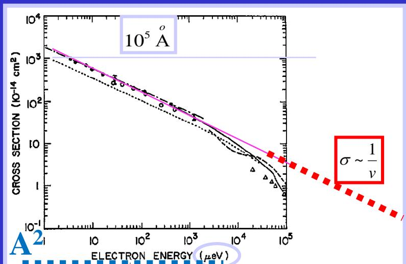
Figure 3. Cross sections for electron attachment to  $CCl_4$ . ●,  $\bar{\sigma}_e$ -K(np); —·—,  $\sigma_e(v)$ -K(np) (Frey *et al* 1994b); ○,  $\bar{\sigma}_e$ -K(np) (Ling *et al* 1992); —, free electrons (Hotop 1994); ---, free electrons (Orient *et al* 1989); △, free electrons (Christodoulides and Christophorou (1971)); ----, theory (Klots 1976).
