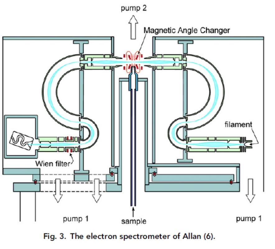
Fig. 3. The electron spectrometer of Allan (6).
