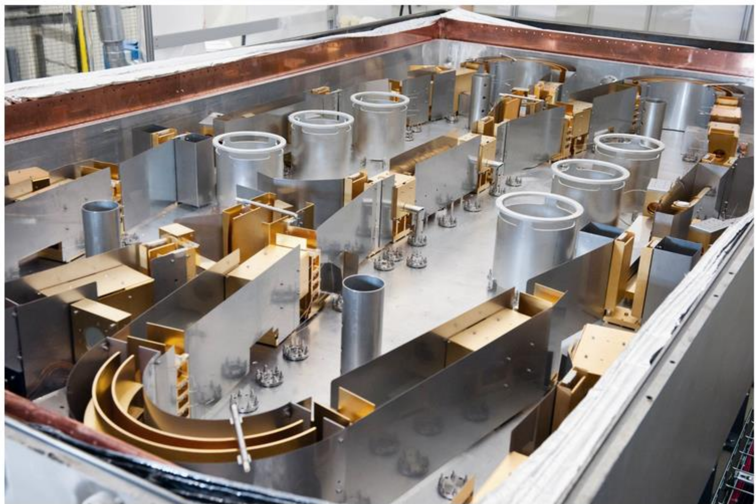
The DESIREE storage rings in their cryogenic enclosure.
