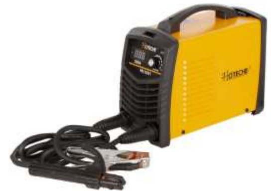
Example of MMA welder with inverter 9 kW, 200 A, 6 kg, 170 EUR
