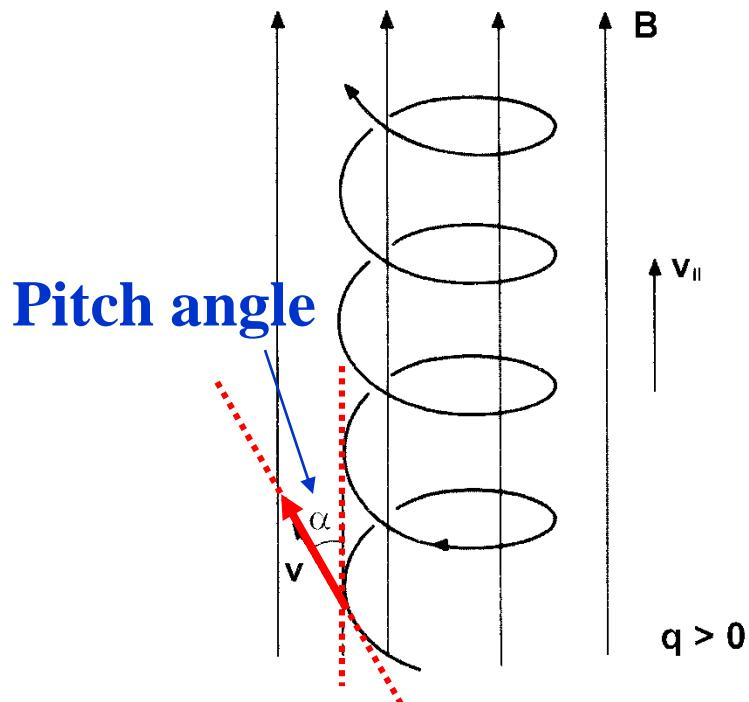
Fig. 3 Helicoidal trajectory of a positively charged particle in a uniform magnetostatic field.
