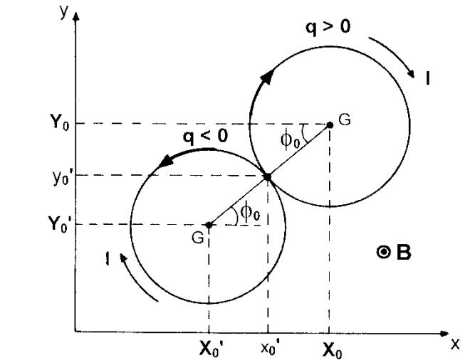
Fig. 4 Circular trajectory of a charged particle in a uniform and constant  $\mathbf{B}$  field (directed out of the paper), and the direction of the associated electric current.
