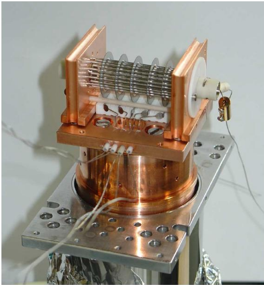
Figure 3.3: The 22-pole ion trap forms the central element of the new ion trap setup. It is mounted on a helium cryostat and can be cooled to temperatures between 8 – 300 K. The base plate of a 50 K thermoshield can be seen, which reduces the heat input on the trap housing caused by blackbody radiation. The 22 rf electrodes are surrounded by five electrostatic ring electrodes, which can be used to shift the stored ions inside the trap. Cylindrical endcaps are used to confine the ions in axial direction.
