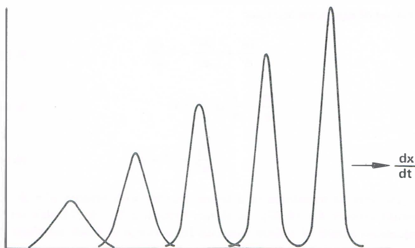
A train of solitons, generated at the left, arrayed according to the relation among speed, height, and width.
