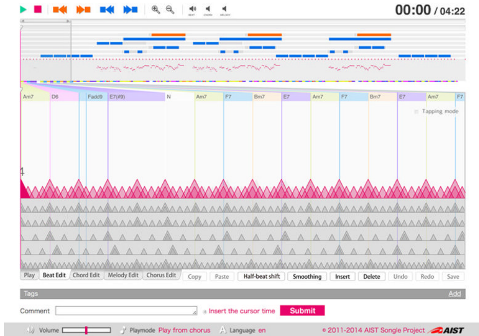
Figure 15.2 A screenshot from Songle, a web service from Japan’s National Institute of Advanced Industrial Science and Technology (AIST). Songle conducts a number of typical MIR sequence-labeling tasks automatically – beat detection, chord estimation, melody extraction, and structural segmentation – and provides an attractive interface for users to view and edit the results (Goto et al. , 2011). Source: http://songle.jp .
