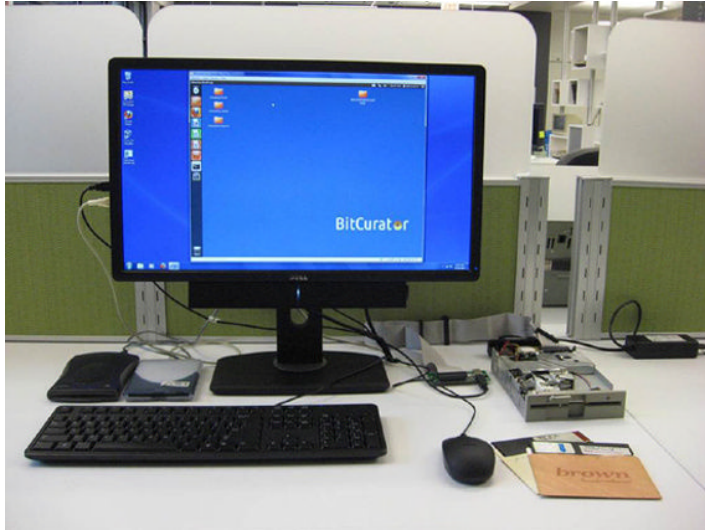
Figure 13.1 Digital forensics workstation at MITH running the BitCurator environment with various media drives, a write-blocker, and a Kryoflux controller card also visible. Source: photo by author.
