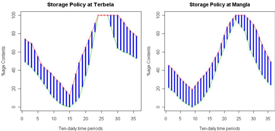
**Fig. 5** Storage level upper and lower limits according to power generation policy i.e. the system will store water into these two storages (Terbela and Mangla) to generate a minimum required power from the system
