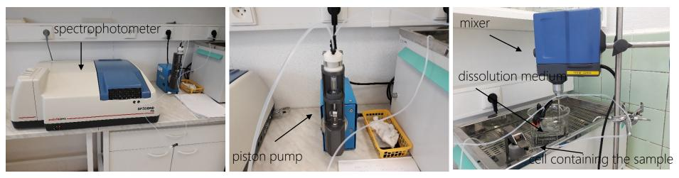
Connection of the tubes (flow-through cell dissolution, close system): medium -> pump > flow-through cuvette -> cell containing sample-> medium
