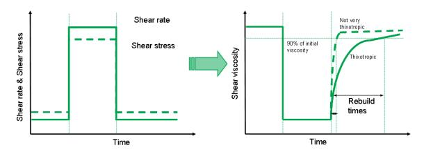
A low shear rate is employed in stage one which is meant to replicate the samples at near rest behaviour. In stage two a high shear rate is applied for a given time to replicate the break down of the sample's structure. The shear rate employed can be matched to the process of interest. In the third stage the shear rate is again dropped to a value generally equivalent to that employed in stage 1 and viscosity recovery followed as a function of time.
