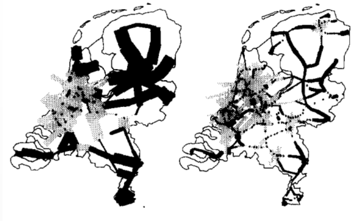
Figure: The line-frequency requirement for Dutch IC/ICE, IR, CT network (1996)
