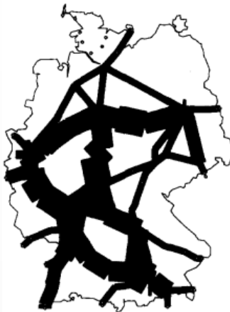
Figure: The line-frequency requirement for German IC/ICE, IR network (1996)
