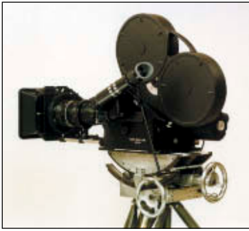
Figure 16.9. The Photo-Sonics 4B, capable of frame rates up to 3250 fps, 100 to 1000 fps in phase lock. (Photo courtesy of Photo-Sonics.)
