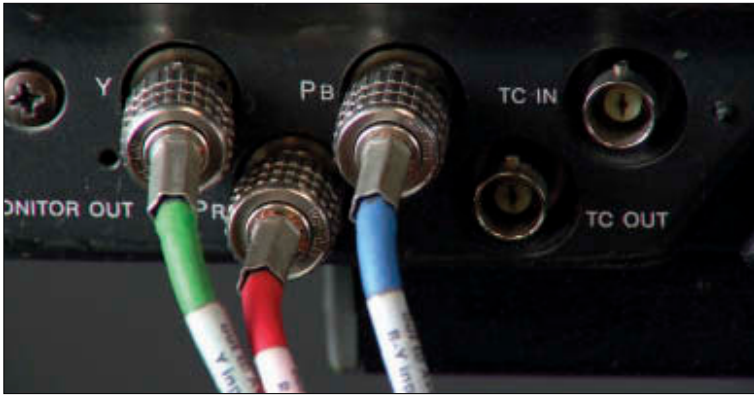
Figure 9.15. Component outputs on the camera: Y, Pr, Pb.
