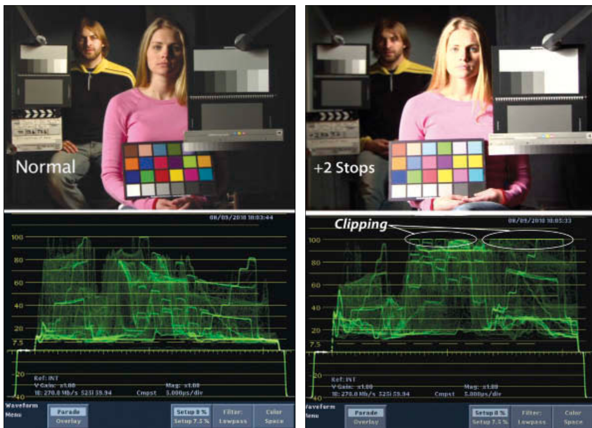
Figure 9.12 (left) Normal exposure on an HD camera. Below it is the same frame on a waveform monitor. Notice the proper skin tones, the correct color saturation in the chart, and how all segments are shown on the gray scale. These images are from a latitude test on an HD camera.
