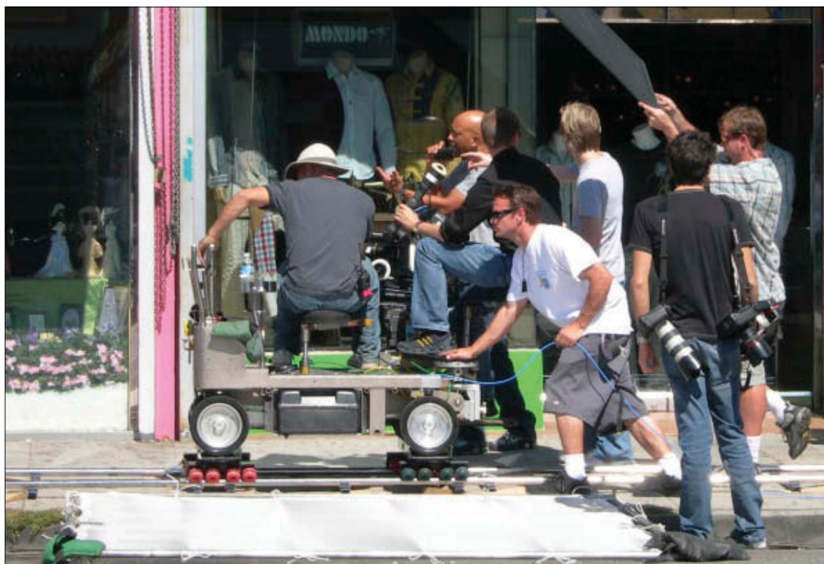
Figure 15.15. Rather than setting the dolly directly on the tracks, many grips use a sled that runs on skateboard wheels; it's fast to set up and more maneuverable. An 8x8 silk is stored temporarily by laying it down and anchoring with sandbags at the corners.
