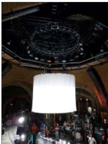
Figure 8.23. An extra-large space light (suspended from the same circular truss shown in Figure 8.20) in a lighting rig designed and executed by gaffer Michael Gallart and lighting director Tony Nako. (Photo courtesy of Michael Gallart.)
