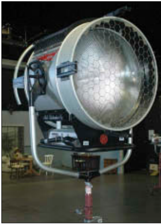
Figure 8.2. (above) A 12K HMI Fresnel.
