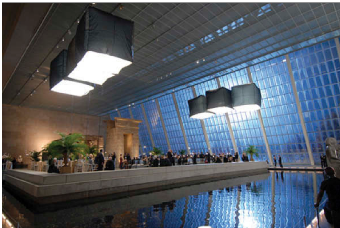
Figure 8.26. Balloon lights require minimal rigging. The museum would have not permitted installation of a heavy-duty lighting grid above the Egyptian temple. In this setup, the balloons have black skirts, which contain and control the spill. (Photo courtesy of Sourcemaker.)
