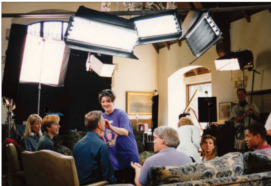
Figure 8.27. Color-correct fluorescents by Kino Flo. Their light weight makes rigging them easier and quicker. Notice how the large window at left rear has been blacked out with a large solid of black duvetyne. A pipe has been rigged to the ceiling to support some of the lights. Note also the snoot boxes on the two tungsten zip lights . (Photo courtesy of Kino Flo.)
