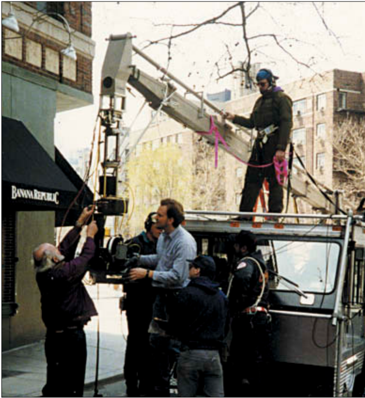
Figure 11.2. A Chapman Lenny Arm rigged on a camera car for some moving shots in Greenwich Village. The grip who will operate it wears a safety harness. (Photo courtesy of Mark Weingartner.)
