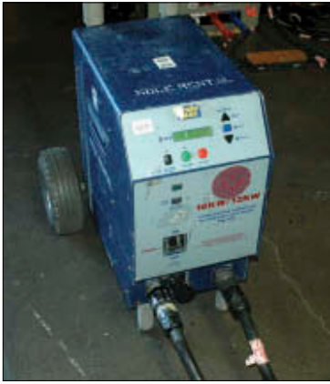
Figure 8.4. (above) The ballast acts as a transformer to provide operating voltage and also starting voltage, which can be as high as 20,000 volts. It is also a current limiter.
