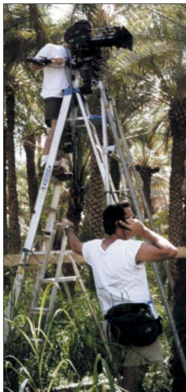
Figure 11.25. Camera on a ladder, one of the quickest ways to get a camera up high. It is usually done with a high-hat clamped and strapped to the top rung. (Photo courtesy of Mark Weingartner.)
