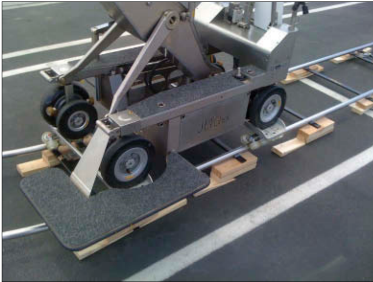
Figure 11.19. (left) A porkchop on a Fisher dolly. The dolly is mounted on a skateboard sled that rides on the tracks.
