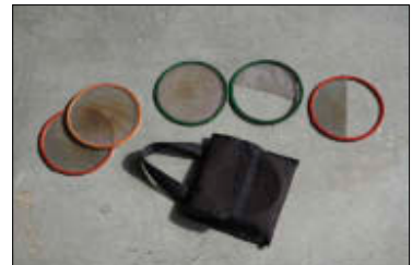
Figure 8.10. A scrim set for a Betweenie . Most lights come with a scrim set to control intensity. A double (red rim) reduces the output by one stop, and a single (green rim) reduces it by one-half stop. Also included are a half-double and a half-single . This is called a Hollywood scrim set because it includes two doubles.
