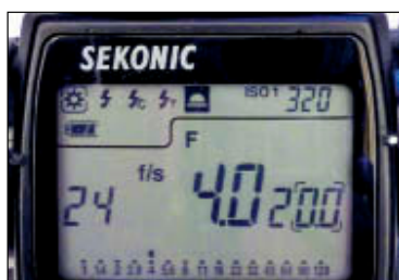
Figure 10.27. (top) A Sekonic Dual-Master light meter. It is a combination of both an incident meter and a spot meter . It can read both continuous light and strobes.
