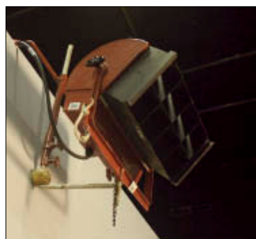
Figure 8.18. (above) A Mole-Richardson 2K Zip Softlight. Zip means it is more compact than a regular softlight. It is mounted on a set hanger (also called wall hanger ). 2K Zips are very popular for just this sort of use: they fit into small spaces and when put up near the ceiling of a set or location, they don't hang down so far that they interfere with the shot.
