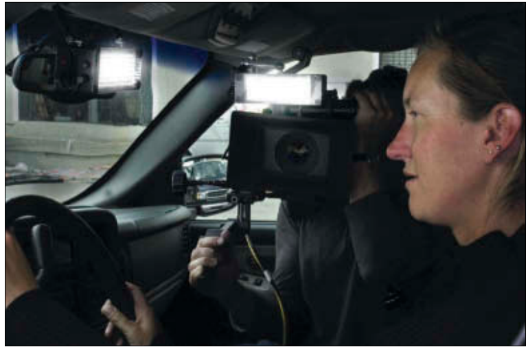
Figure 8.7. Lite Panel LED lights mounted in a car and also as a fill light on the camera. This type of camera mounted fill light is called an Obie , named for actress Merle Oberon, for whom it was invented. Due to their light weight, compact size and, ability to run off batteries, LED units are very popular as camera mounted lights. (Photo courtesy of Litepanels.)
