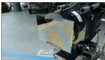
Figure 15.5. (top) Attaching a filter to a lens when there is no matte box or the filter won't fit the matte box can be accomplished by making a daisy out of camera tape (1 inch cloth tape).
