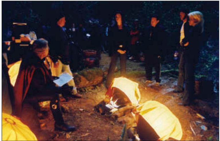
Figure 15.18. Chief Lighting Technician Tony Nako (standing at left) setting muzz balls for a fire effect on X-Men II . (Photo courtesy of Tony Nako.)
