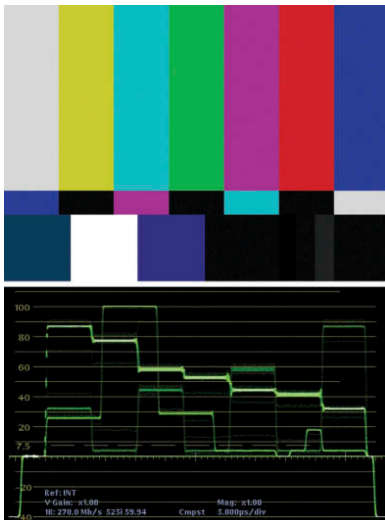
Figure 9.7. (top) SMPTE 75% color bars as they are seen on a video monitor. The primary and secondary colors are arranged in order of brightness. On the far left top is a 75% gray patch. In the bottom row, second patch from the right is a 100% white patch. (bottom) The color bars as seen on a waveform monitor , which measures the voltage of the video signal. Also on the lower row at the right on the color bars is the PLUGE, which can be clearly seen on the waveform signal.
