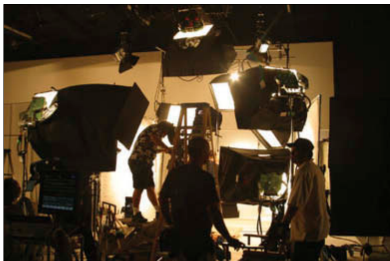
Figure 8.21. (top) Barger Baglights with Chimera softboxes in use on a hair product commercial. The reason there are so many lights is that they are dimmed up and down for different shots or when the model moves. Also, since this is a hair commercial, light coming from any directions makes for more reflections and sheen on the hair so it looks its best. This is a key advantage of tungsten lights: they can be controlled from a dimmer board. In comparison to a 5K with a Chimera , the Bargers have wider, more even throw and take up less real estate on the set.
