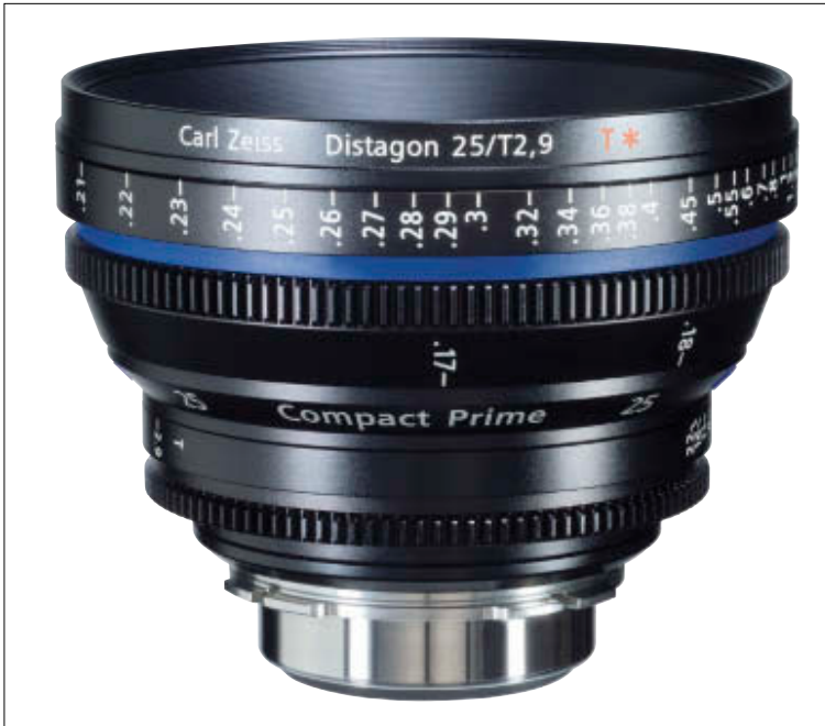
Figure 14.3. A prime lens has only one focal length, unlike a zoom, which is variable in focal length. This lens is a 25mm T/2.9 by Zeiss. A lens is defined by its focal length and its maximum wide open aperture. (Photo courtesy of Carl Zeiss AG.)
