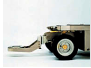
Figure 11.19. (left) A porkchop on a Fisher dolly. The dolly is mounted on a skateboard sled that rides on the tracks.
