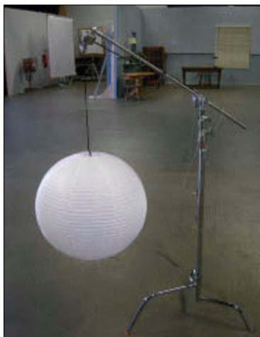
Figure 8.24. A China ball suspended from a C-stand. These are a cheap and extremely lightweight source of softlight and are easily rigged.
