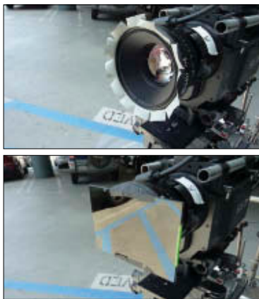
Figure 15.5. (top) Attaching a filter to a lens when there is no matte box or the filter won't fit the matte box can be accomplished by making a daisy out of camera tape (1 inch cloth tape).
