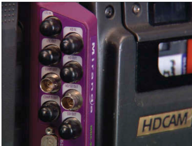
Figure 9.16. HD SDI outputs, as well as composite, timecode, and other connections on a Miranda downconverter.
