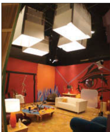
Figure 7.16. (top) This rig by Tony Nako for X-Men uses dozens of Kino-Flo units to create a soft overhead ambient light to suggest an overcast winter day.
