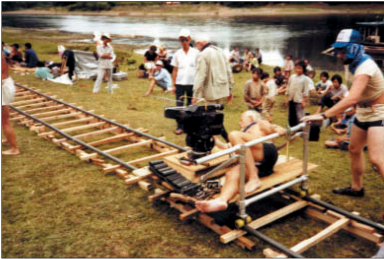
Figure 11.3. A very simple pipe dolly rig for this Imax shot in China. Pipe dolly rigs are especially useful for situations like this where a rental dolly is unavailable and it is impractical to fly one in. Many people carry the wheels and hardware with them and build the dolly and track with locally available materials. (Photo courtesy of Mark Weingartner.)
