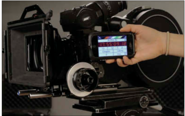
Figure 15.12. Timecode slating with an iPhone. The camera being photographed is a 35mm Arri BL4. There are several excellent timecode slate apps for smart phones and notepad computers.
