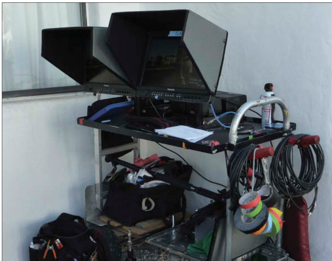
Figure 15.19. Video village on a two-camera HD shoot. The monitors are mounted on the camera assistant's Magliner Junior , which makes moving them quick and easy.
