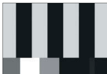
Figure 9.17. Blue-only color bars shown in black-and-white for clarity. Notice that the bands are of equal intensity, and in the upper portion the large and small bars are equally gray or black. This indicates correct phase and saturation.
