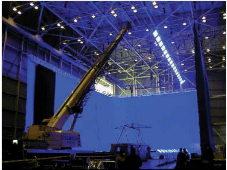
Figure 16.8. A very large blue-screen setup: there are rows of Kino Flo units rigged from above and another row near the floor. (Photo courtesy of Kino Flo.)
