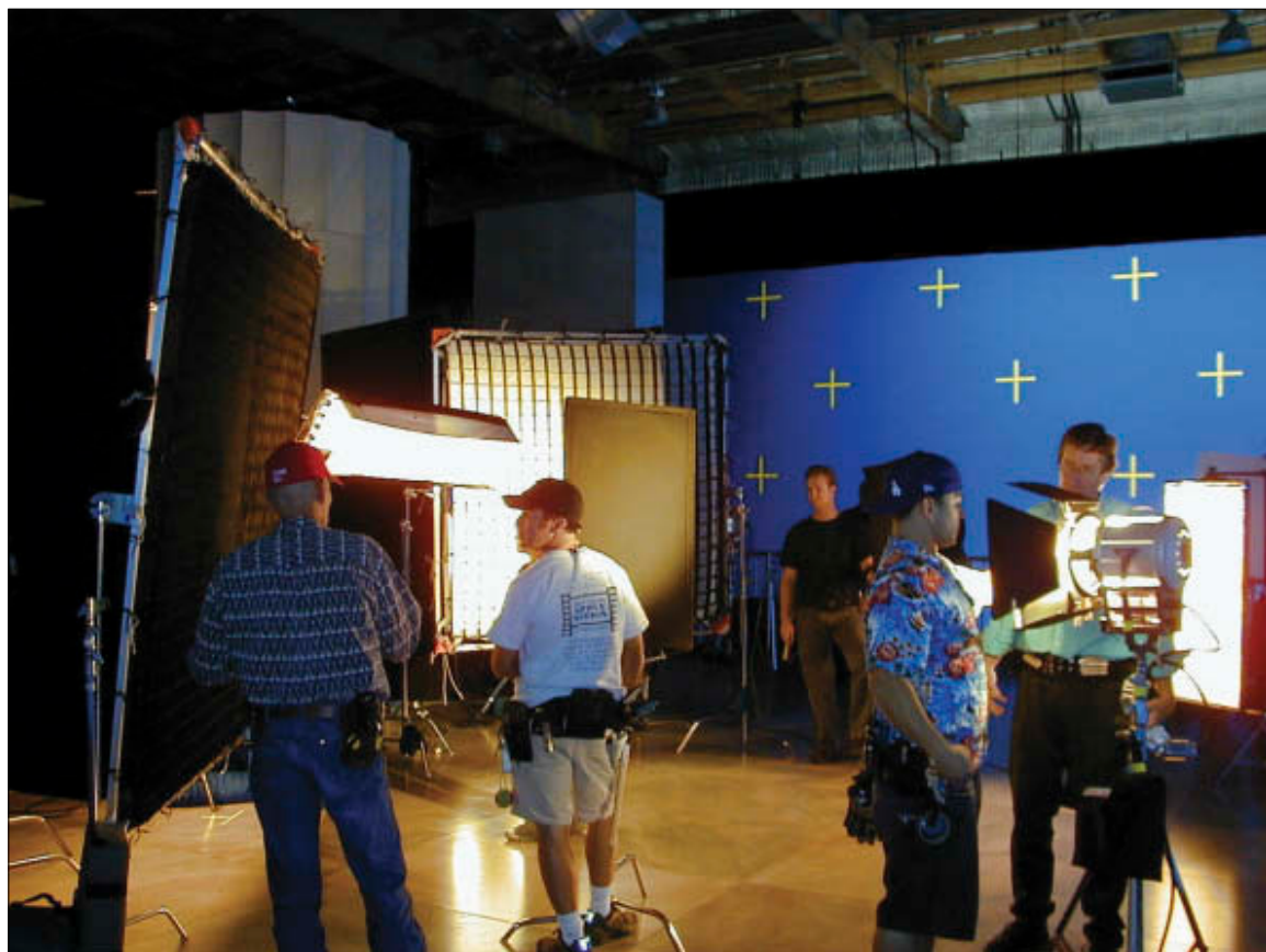
Figure 8.3. A combination of Kino Flo and tungsten units on a blue-screen efx set. (Photo courtesy of Kino Flo.)
