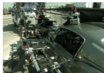
Figure 11.24. A fully tricked out car rig with camera mounted on a hostess tray on the driver's side for running shots.
