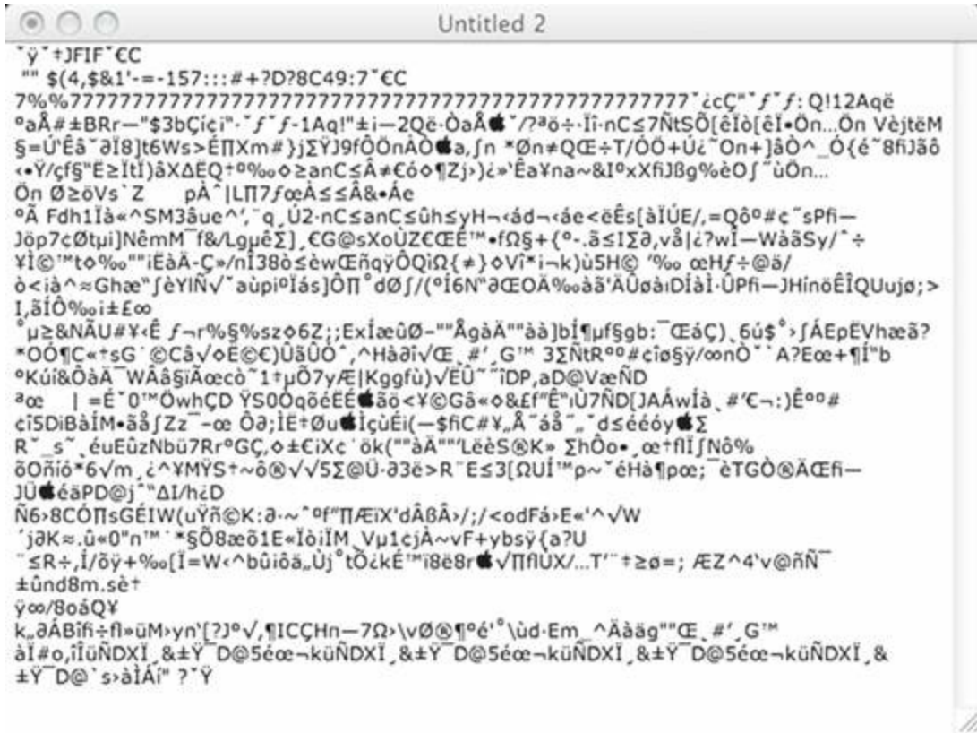
Figure 3.4. Image of a red circle saved as .txt and opened in a text-editor
