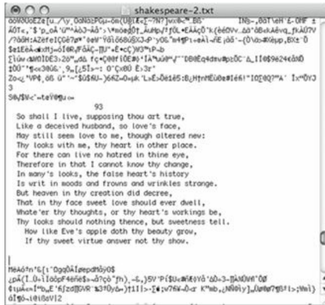
Figure 1.2 . Inserting Shakespeare’s 93d sonnet three times into the source code of an image.
