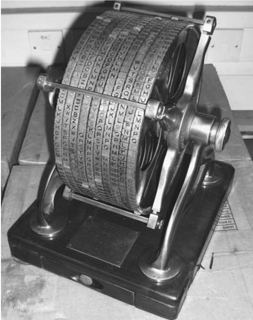
Figure 5.6 Joseph Grassi's machine for producing pronounceable code groups. Photograph by Nicholas Gessler.
