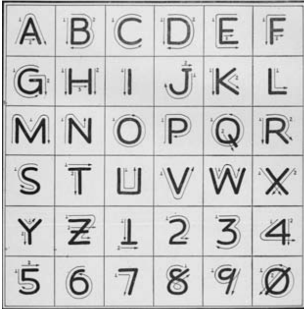
Figure 5.2 Army chart (1945) showing the directions in which letter strokes should be made. Photograph by Nicholas Gessler.
