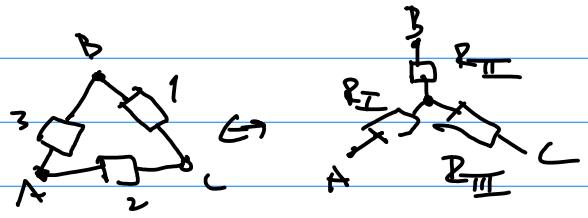
$$\frac{1}{R_1+R_2+R_3} = R_I + R_{II}$$
