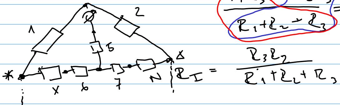
$$\frac{R_1 R_3 + R_2 R_3}{R_1 + R_2 + R_3} = (R_I) + (R_{II})$$
