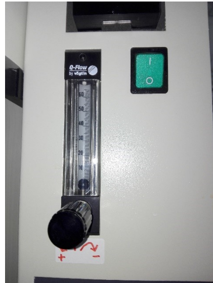
Fig. 2: Rotameter for the air flow setting
