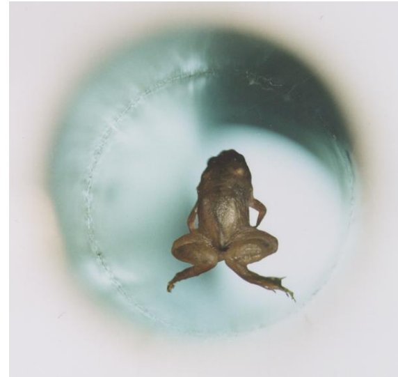
A live frog levitates inside a 32 mm diameter vertical bore of a solenoid in a magnetic field of about 16 T
