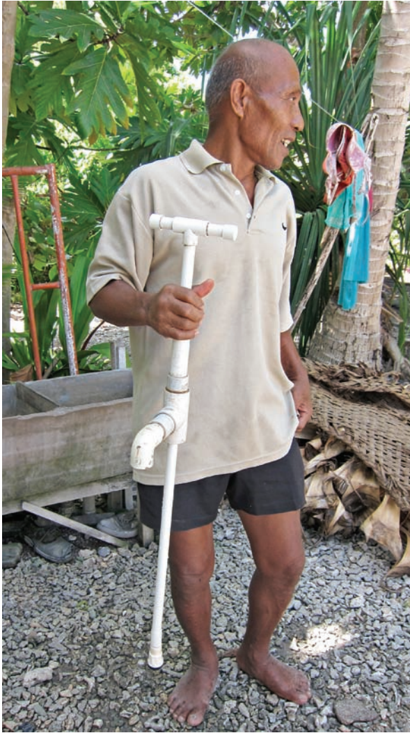
The Tamana water pump – a local invention made partly from waste.
