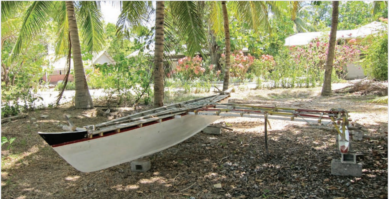
The traditional I-Kiribati canoe is tied together with coconut string.
