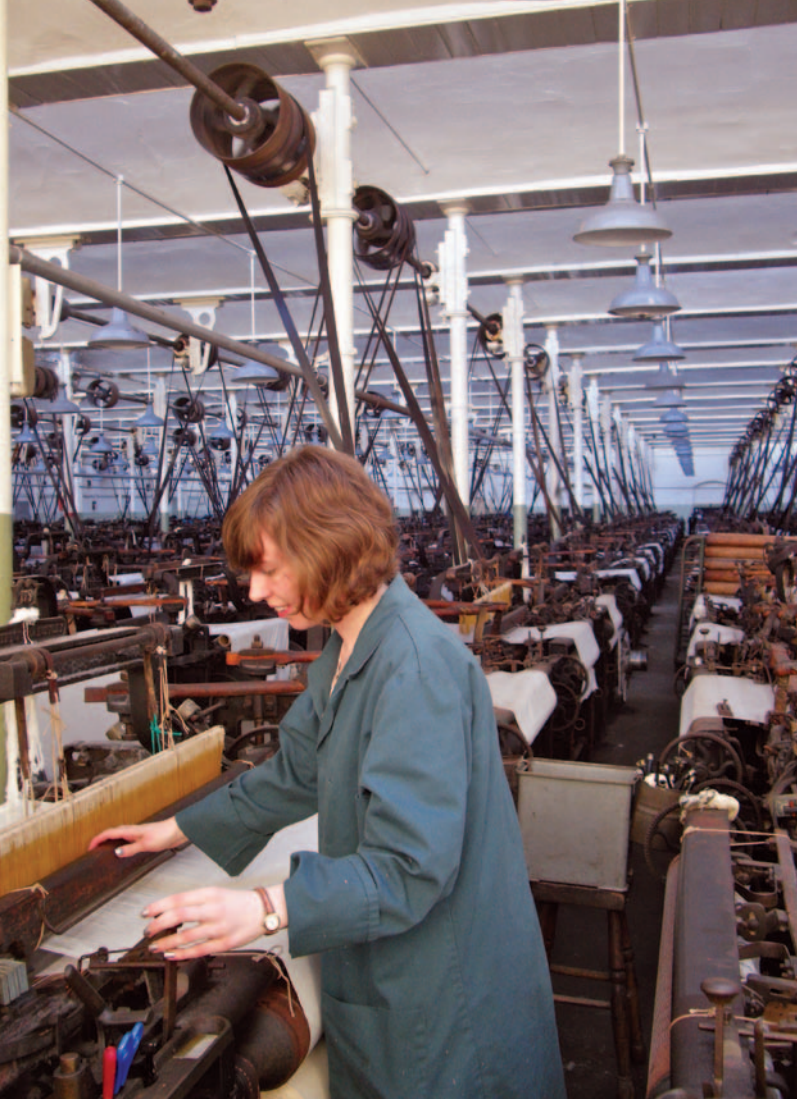
Queen Street Mill, Burnley, England. This once-typical weaving shed from 1894, its looms powered by a Lancashire steam mill engine through line-shafting and belt-wheels, is now unique and preserved as a working cotton mill. The accident of survival has made this a site of outstanding importance. (Neil Cossons)
