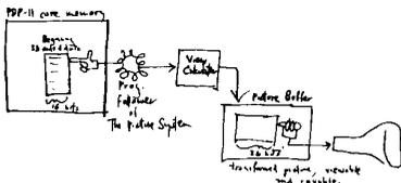
Another important feature of The Picture System: it will do, not just ordinary perspective, out such weird view calculations as wideangle barrel distortion, pincushion distortion and similar stuff.
