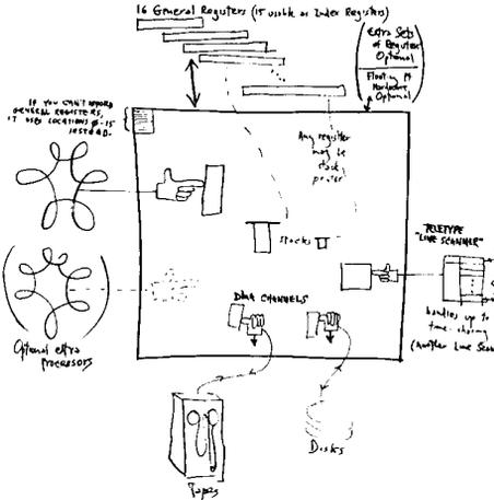
The PDP-10 has 36 bits but has instructions to operate on chunks, or bytes, of any length. It has sixteen main registers, as does the 360, but uses them more efficiently.
