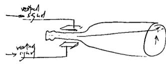
the horizontal deflection plates can pull the beam sideways on the screen, controlled by a signal to them.
