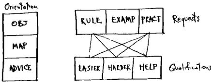
What I am trying to show here is that merely the arrangement of buttons creates different fancic constructs. If you see this, you will recognize that considering all the other options we have, designing new media is no small matter. The control structures merge mentally with the presentational structures. The temptation to settle on short-sighted designs having shallow unity is all too great.
