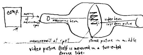
I have heard it said that it might be possible to build a CRT with a changeable mirror surface: that is, the screen becomes mirrored temporarily where it is being hit with the electron beam. Interesting. This would mean that you could make computer displays (and TV) bright and projectable to any degree, say, by pouring a super-intensity laser beam on it. "Be great for writing 'Coca-Cola on the moon," said a friend of mine. If you believe in astral projection.
