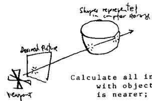
Calculate all intersections of sighting ray with objects in scene; calculate which is nearer; shade it according to angle.
