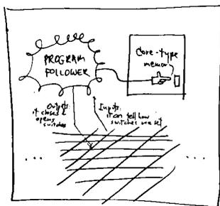
Depending on the numbers that have been dialed, and whatnot, the ESS jumps to a specific program, and that tells it to connect an incoming call to particular other circuits, or to ring other lines, or whatever.
