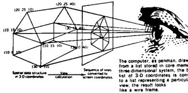
The computer, as penman, draws lines from a list stored in core memory. In a three-dimensional system, the basic list of 3-D coordinates is converted to a list representing a particular view; the result looks like a wire frame.
