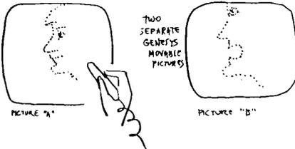
Now, to create the animation, you do the same thing. Each image can be made to move on the screen; and the path of the motion may be drawn on the screen, through the picture area. Not only that, but the timing of the motion is controlled through the same diagram, by the spacing of the dots. (Baecker calls his control diagrams p-curves.)
