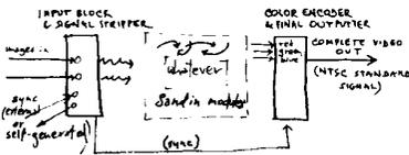
For the sake of clarity we will refer to the outputs as pictures, or as black, white or grey, which they would be if they went straight out to a screen; but they may be turned back into the system and function as inputs as well. "White" means +5 volts, "black" means -5 volts.
