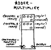
The channel A inputs are added together and multiplied by C; the channel B inputs are added together and multiplied by the reverse of C; both results are added to make the output. (NOTE: this unit is used among other things, for fades and keying.)
