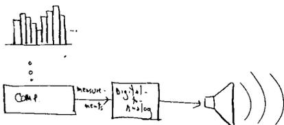
In the easiest case, the computer can just send back out the voltages it originally got in. This is rather ridiculous— using the computer just as a recording device— but it's a clear and simple example.
