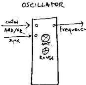
The two planned uses were A) with a sync, to generate fixed patterns, and B) without a sync, to generate movable patterns. If both inputs are used, it becomes a stubborn lock-on voltage-controlled oscillator, which tends to grab at passing submultiples.
