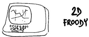
A surprise something-or-other from DEC, the VT55, represents a breakthrough of some sort. But what were they thinking of? "Graphic capability" has been added to an ordinary upper-case keyscope. Specifically, the ability to make two graphs, i.e., two wiggly lines (no score) somewhere between the left and right sides of the screen. You can also shade in under them, and add coordinate grids. It's \$2500, and obviously great if you're bonkers for 2D graphs.
