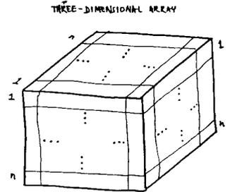
A one-dimensional array is like a row, a two-dimensional array is like a tabletop, a three-dimensional array is like a box, and for more dimensions you can't visualize.
