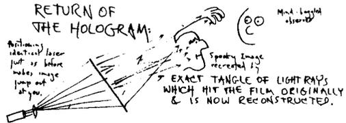
Diagram of how hologram is made, p. DM 20.
