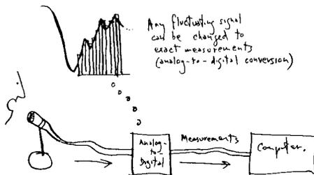
To make sound by computer is the obverse. If the computer can be set up to send out a string of measurements, these can be turned back into a fluctuating voltage, and thus make sounds.
