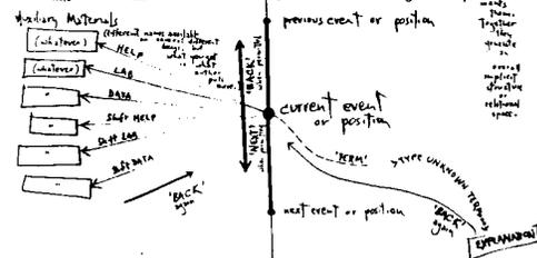
The original idea was evidently that there would be a basic sequence, in which NEXT and BACK would be the forward and back controls, and the other six would represent help for the Confused, a "tab" allowing experiments, and additional data the student decides he needs. The three with Shifts simply provided a second option of each type.
