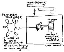
Well, a microprocessor has two levels. It has an upper-level program follower with its own binary program. But each instruction of this upper-level program is in turn carried out by a program follower running a program at a lower level — called a microprogram.
