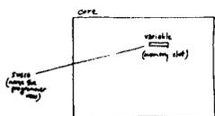
An **array** (also called a **table**) is a section of core memory which the programmer cordons off for the program to put and manipulate data in. If SPENCER is the name of the array, then SPENCER(1) is the first memory slot in it, SPENCER(2) is the second, and so on up to however big it is.
