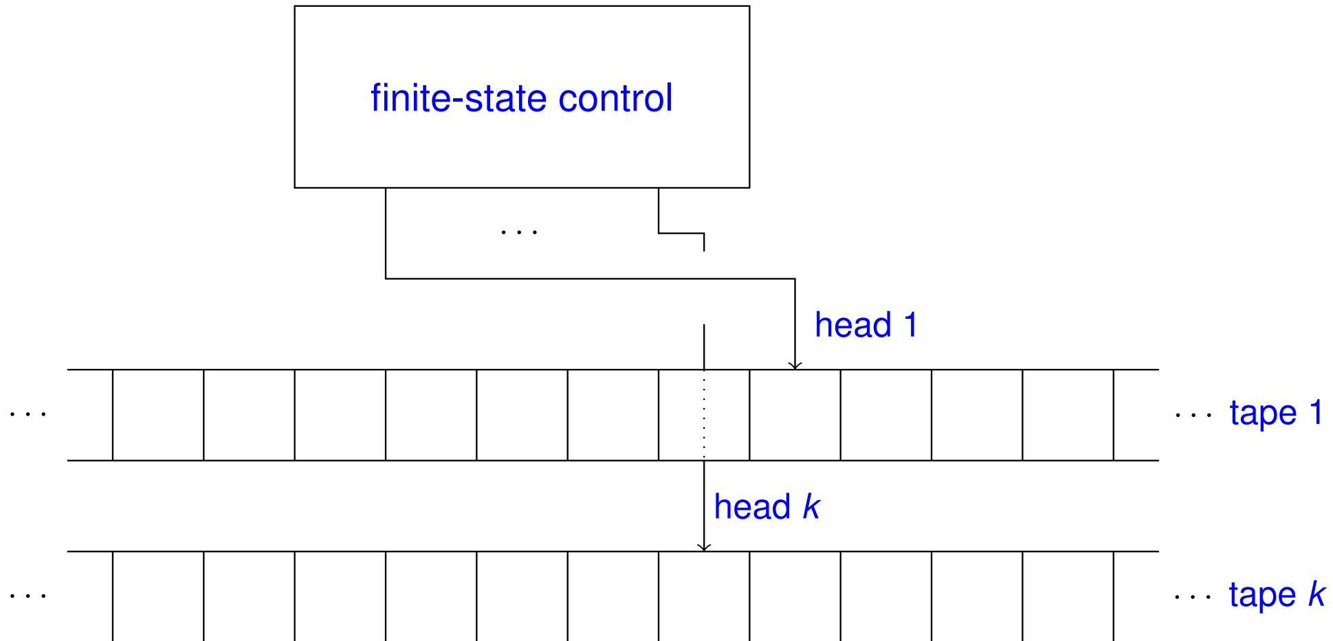
Formally a **Turing machine** (TM) with  $k \geq 1$  tapes is defined through a 7-tuple  $M = (Q, \Sigma, \Gamma, \square, \delta, q_0, q_1)$ , where
